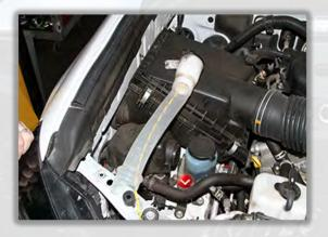
Next loosen the 4 bolts holding on the radiator to the sub-frame- (2 upper and 2 lower). Let the radiator loose and rest on the frame.
