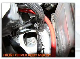
Remove the clips holding the inner rubber fender liners by the front wheel wells, from the frame side on both sides. Each bolt that is connected to the frame has a washer with a notch attached to the bolt, you will need to twist to remove the bolt.
