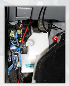
For the body mounts in the middle, take off the plastic trim on the sides of the rear seats. Lift up the carpet and you will see the hole that leads to the body mount in front of the rear tire.
