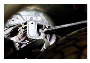
5) Access all of the body mounts and loosen them, removing 3 of the bolts on one side at a time. The 2 front mounts are located behind the front bumper. (shown in pic below with extension attached)
