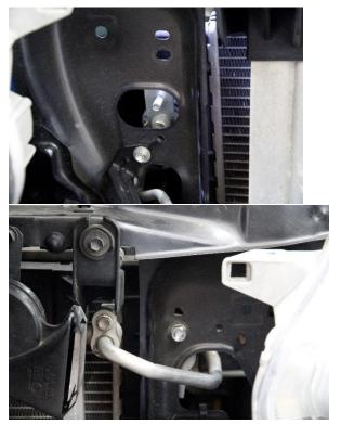
11) You can reinstall the grill and radiator cover. The radiator cover will not clip back onto the radiator.
