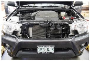
3) Remove the 4 radiator bolts to the body - (2 upper and 2 lower). Let the radiator loose and rest on the frame.
