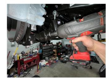
5.Remove the lower strut mounting bolt and hardware from the lower control arm. **Note: this is the last part holding the lower control arm from swinging down out of the way, Carefully remove bolt so that no damage or injuries can occur.**
