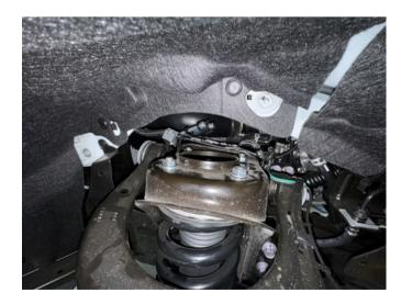
10.Using a pry bar or similar tool that will fit in the lower eyelet of the front strut, carefully turn the body of the shock so that it will line up with the lower mounting pocket of the lower control arm.
