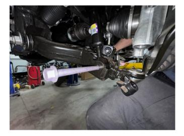
12.Re-install the 2 lower ball joint mounting bolts to the bottom of the steering knuckle. Torque to 150 ft lbs.
