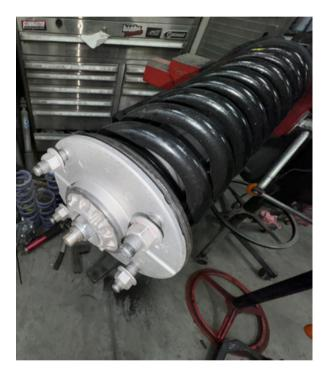
7.Thread the OE nuts on to the studs of the strut and Measure 3/8" from the tip of the studs down, make a mark and using an appropriate cut off tool, cut the OE studs. Once threads have been cut, remove the OE nuts and this will clean the freshly cut studs.
