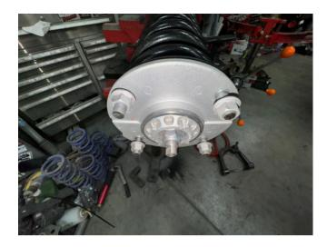
8.Locate and install one of the new upper strut spacers on the top of the OE strut using the OE nuts. Note: The spacers will only fit on the strut one way, if the bolt pattern does not line up, rotate the spacer until it does. Torque OE nuts to 40 ft lbs.
