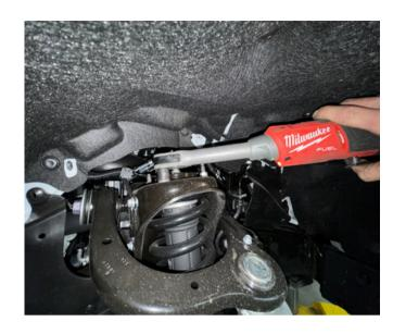
2. Loosen, but DO NOT remove the Lower control arm mounting bolts.
