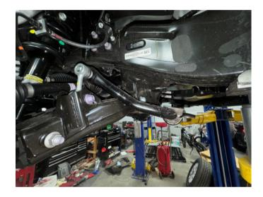
4.Working on the driver side, Remove the (2) bolts holding the lower ball joint mount to the knuckle. Save hardware
