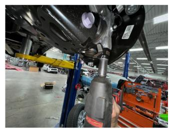
13.Move back to the 4 new 3/8" flange nuts on top of the strut and torque to 40 ft lbs.
