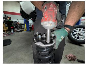
9.Re-install the strut to the vehicle using the new 3/8" flange nuts, Leave loose for now.
