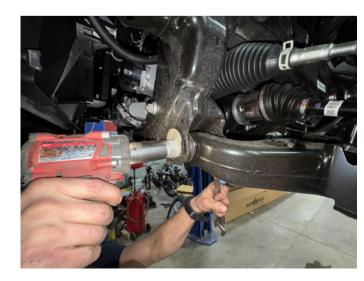
3.Remove the sway bar mounting bolts on the driver and passenger side frame. Let the sway bar hang loosely.
