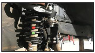
19. Move back to the 9/16" x 5" bolts and tighten to **125 ft**
