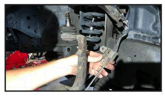
7. Remove the rubber grease boot from the upper ball joints,
