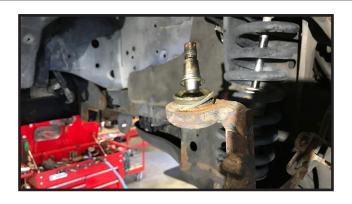
Using an air hammer or ball joint service tool, carefully remove the upper balljoint from the steering knuckles.
