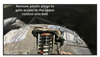
11. Remove the upper control arm bolt. Special note: some vehicles may have a wire harness that is attached to the inner fender that could obstruct the bolt from being completely removed, if you run into this, you will need to unbolt the wire harness bracket temporarily to gain room to remove the bolt.
