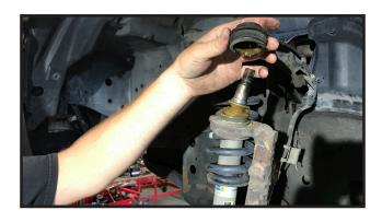
8. Remove the snap ring from the upper ball joints
