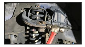
6. Locate and remove the bracket holding the ABS wire to the very top of the steering knuckle
