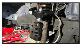
18. Now locate the 5/16" x 1 1/4" x 2" round u-bolts, and 5/16" flange nuts. Install the u-bolts around the neck of the steering knuckle and through the support bracket mounting holes. Do not tighten the 5/16" flange nuts yet.
