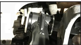
16. With the new upper control arms installed, Locate the S10335 uniball adapter sleeves from hardware bag 50965NB. Install these into the top of the steering knuckles where the OE ball joints were removed from. Note: It may be necessary to us a file or similar tool to clean up the inside of the OE ball joint hole at the top of the knuckle.
