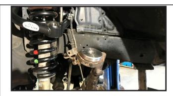
17. Using the photos below as a guide, locate the S10246 uniball mis-alignment sleeves, 9/16" x 5" bolts, 1/2" flat washers, 9/16" unitorque nuts, knuckle support brackets, and install the upper control arms to the steering knuckles. Leave the 9/16" bolt and hardware loose for now.
