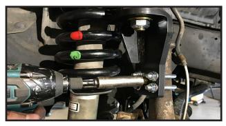
22. Re-install the ABS wire harnes bracket over the welded on bolt on the new upper control arms. Secure using the new 1/4" nut, and 1/4" flat washers from hardware bag 50965NB.
