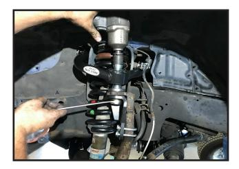
20. Now you can tighten the 5/16" flange nuts so that it closes the gap between the knuckle support bracket and the neck of the steering knuckle.
