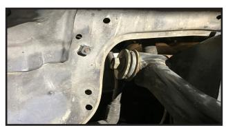
12. Once the bolt has been removed, go ahead and remove the upper control arms from the vehicle.
