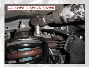
11. Being careful not to overextend and pull apart the inner CV Axle joint, move the spindle/hub assembly out of the way so the coilover can be removed from the vehicle. Remove the coilover on both sides.
