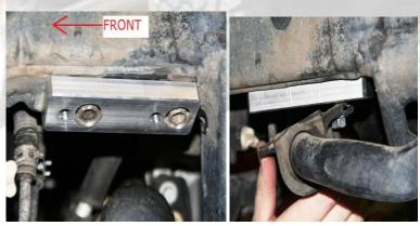
14. Reinstall the lower ball joint bolts, wheels/tires, and the skid plate. Torque all bolts/nuts to manufacturer specs.
