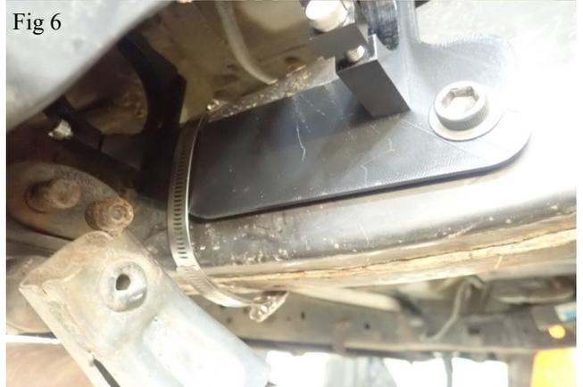
Install lower mount first onto the axle, then compress shock to slide upper stud into place.
