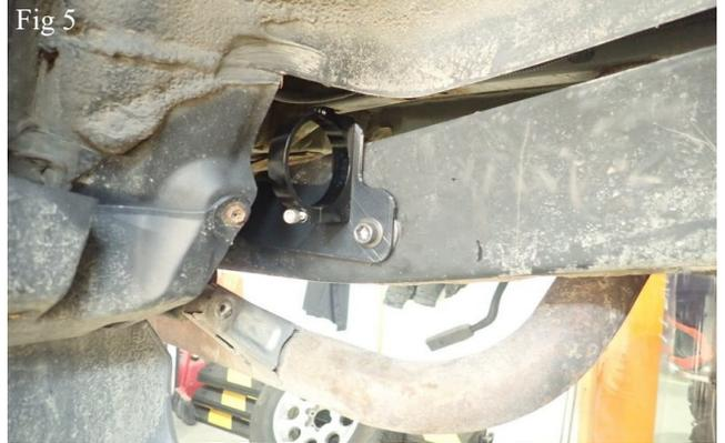
Once bracket is bolted down, use the supplied steel collar around the frame and resi mount. Be careful to not place the collar screw where the resi will be installed.
