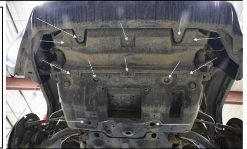
**#2** Support the differential with a floor jack or transmission jack.
