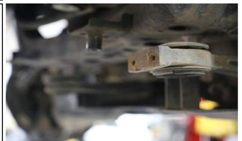
**#4** Lower differential far enough to allow insertion of the 1" drop spacer
