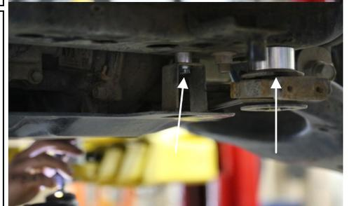
**#6** Install the front skid plate using the OEM bolts on the front part of the skid plate and the supplied longer bolts with washers and circular skid spacers on the rear portion of the front skid.
