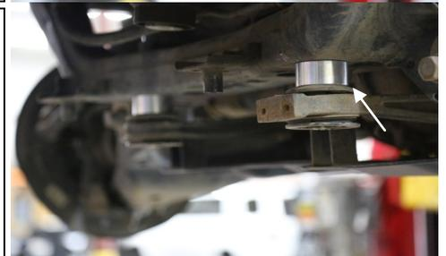
**#5** Install the 1" spacers between the two front differential supports and front cross-member. Fasten to cross-member using new 1/2" x 6" long Grade 8 bolts and nuts (making sure to reuse the factory washers). Tighten to the factory specifications. If you don't have the factory specs, 50-70 ft.lbs. should be adequate for this size/grade bolt.
