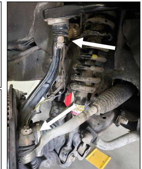
**#4** Now that you have room to remove the strut take the tops nuts off completely and swing the lower part of the shock down towards the front of the vehicle out of the LCA shock ears. Once it is down to the side you should be able to slide the top studs past the frame mount and remove the strut from the vehicle.
