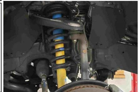
**#3** Once the bolts and nuts are loose proceed to remove the lower shock bolt.
