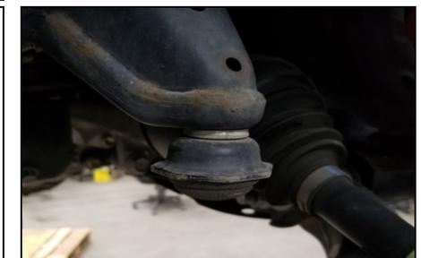
**#5** With the strut out it is now very easy to get to the front and rear bumpstops so go ahead remove those and install the bumpstop drops. When re-installing we like to use a little bit of anti-sieze in case you ever want to upgrade your bump stops. It also a good time to install UCA's if you have them.
