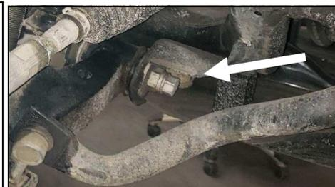
**#6** Now to install the new coilover it is easiest to bolt up the top loosely so you can manipulate the bottom end. Once the top is in place you may need to pry down a little on the lower control arm to get the lower bolt through the arm without damaging the threads.
