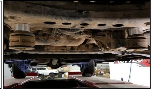
**#8** Now that front end is installed retorque everything you touched back to factory spec except for the lower shock and the cam bolts. These need to be tightened with the weight of the vehicle on the ground after a couple of jounces. Also wait until the vehicle is on the ground to reconnect the sway bar.
