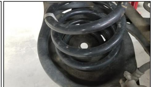
**#11** For the next step you will need a special coil compressor from oem automotive tools. This will allow you to compress the rear coil safely from inside of the coil for installation as the lift springs are quite a bit more stout than factory. We recommend to slip the drivers side trim packer in to help with drivers side lean.
